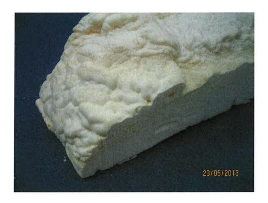
Determination of declared value of thermal conductivity  $(\lambda_D)$  of SEALECTION Agribalance® two component open cell, spray applied, semi-rigid polyurethane foam
