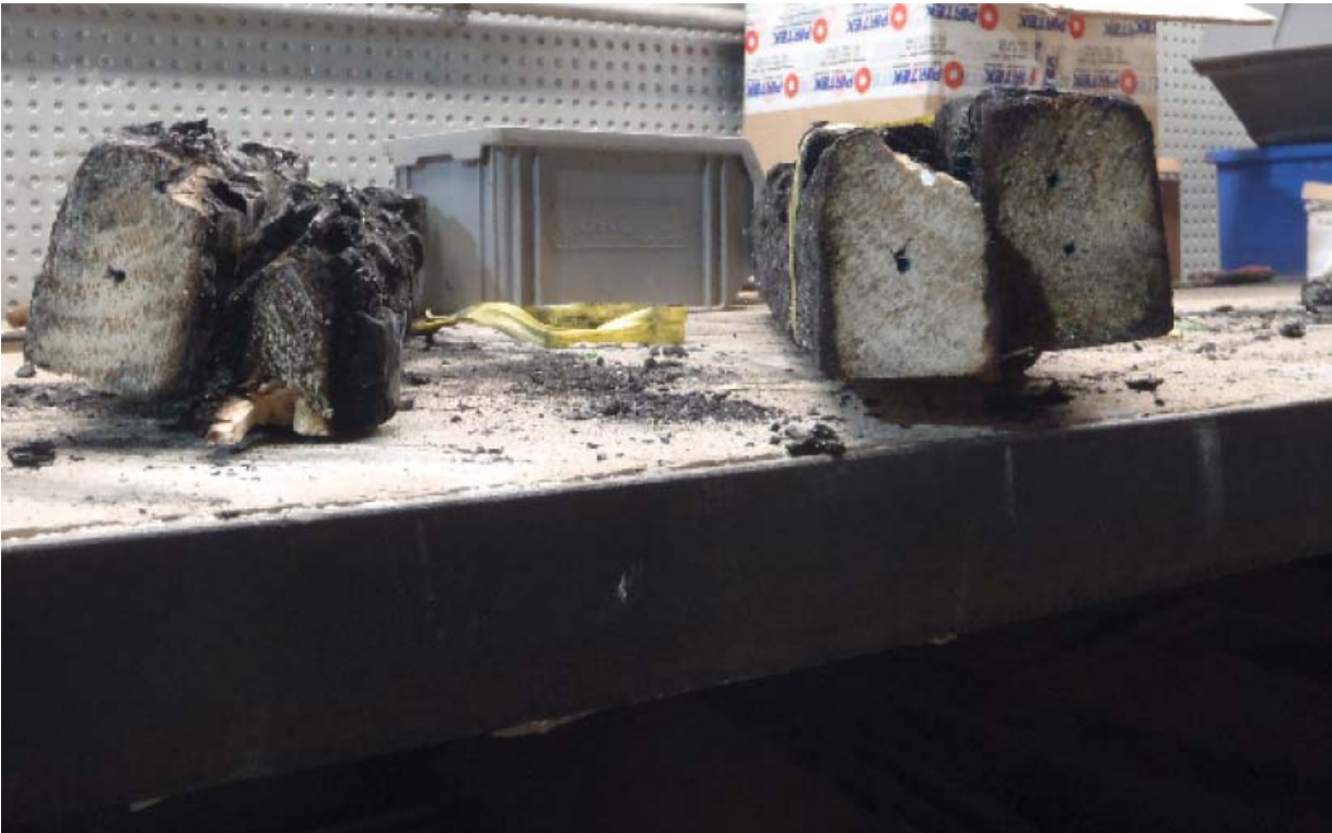
Samples of timber after the test – the specimen with foam in the cavity on the right.
