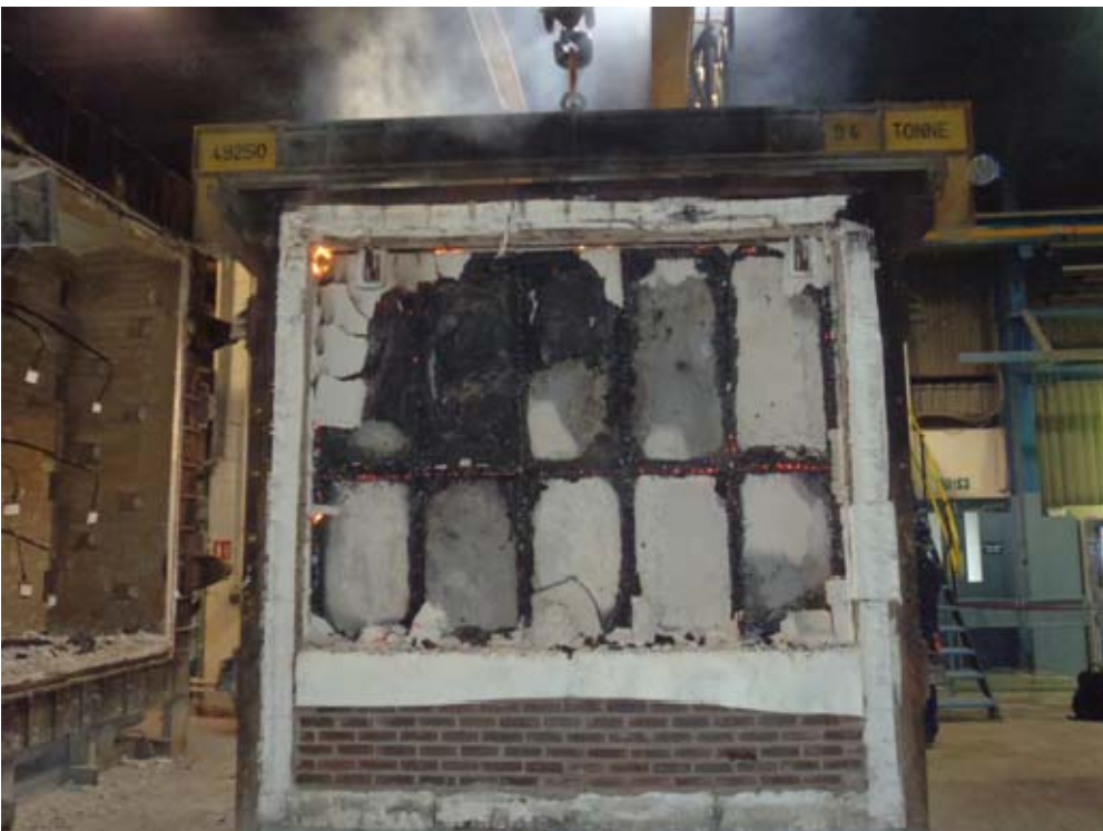
The exposed face of the specimen (with foam in the cavity) immediately after the test
